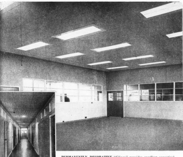
**PERMANENTLY DECORATIVE** "Glinex" provides excellent acoustical correction and absorption, as well as thermal insulation. It is permanently decorative and can be used as a core (faced with wood veneers, asbestoscement, hardboard, kraft paper, etc.) or used in its natural state. Uses include roofs, walls, partitions, ceilings, doors, sub-floors and fitments. Available in 9 thicknesses and 5 densities. 5 standard sized panels.
