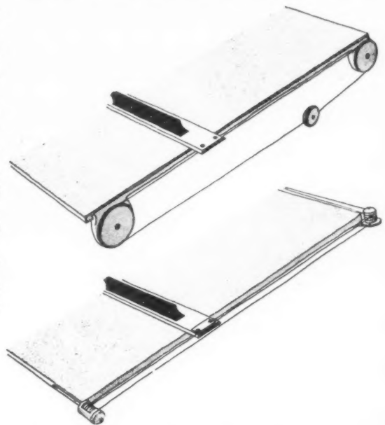
Fig. 7 (left). Adjustable angle-iron frame support. Fig. 8 (top). Counterweight type of parallel motion. Fig. 9 (above). Spring wire type.
