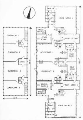
Ground and first floor plans, house blocks A and B [Scale:  $\frac{1}{2}b^{\prime\prime}=1^{\prime}\,0^{\prime\prime}]$
