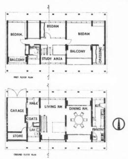
Fig. 14: ground and upper floor plans of the Esso West Africa grade 2 house.
