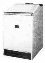
Burner and controls are totally enclosed in the 'Potterton' 70; it is designed for use with 35 sec. domestic fuel oil and has an output of 70,000 B.t.u/hr.
