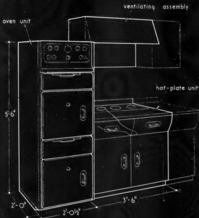
ER.94 REVO ELECTRIC COOKER, SHOWING VENT-AXIA VENTILATING ASSEMBLY.
