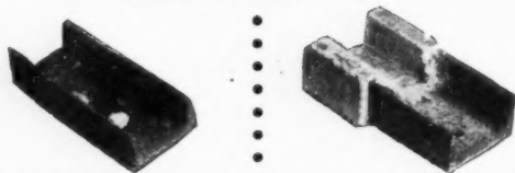
The photograph on the right shows the complete protection offered by Sprayed 'Limpet' Asbestos against corrosion. Both channels were subjected to the same conditions, the test being carried out in a dyeworks.
