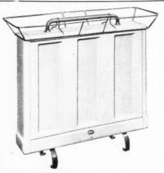
MEMRAD RADIATOR has tubular heating element with baffle plate which disposes heat evenly over casing. Plastic covered lifting handle. Mushroom body with alternative red or brown lifting handle and feet. Rating 1 kW. Chrome detachable rail for drying clothes can be supplied as an extra.
