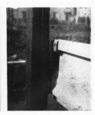
Fig. 21 (left), spring-loaded wind bracing unit on test structure. The spring is in compression allowing bracing unit to lengthen as the jack below the stanchion on left is lowered. Fig. 22 (centre), testing timber window for "lozenging." The window is 10 ft. wide × 8 ft. high. It is fixed rigidly to the stanchion on the right. The jack on the left has raised the left-hand side of the window 3 in. No
