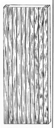
The MERIDIAN door has shallow "V" grooves it wide at intervals of 3" across each face. It can be stained, varnished or painted, and is available with glazing openings if desired. Both internal and external doors are offered.
