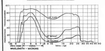
Fig. 7, energy transmission curves for normal plate glass and for two heat absorbing glasses "Antisun" and "Calorex." Note that though both the latter give relatively high transmission in the visible range, they show a dropping off at the red end of the spectrum to give the characteristic blue-green colour.
