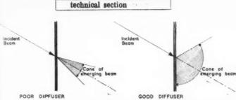
Fig. 2, diagrams illustrating the operation of diffusing glasses. The wider the cone, the better the diffusion.
