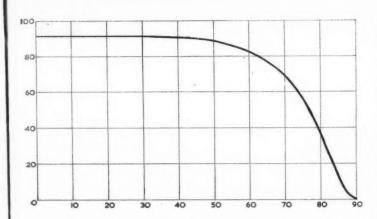
Fig. 1, graph showing the variation of light transmittance according to the angle of incidence of the light for a glass of refractive index 1.5. The vertical readings are percentage transmittance, the horizontal readings are angles of incidence in degrees. Note that there is no significant drop in transmittance ut to an angle of 45°.
