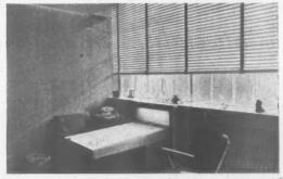
View of Director's Office : Insulated double-wall Compactite partitions faced with Etchwood; desk and filments designed and constructed by Compactom.
