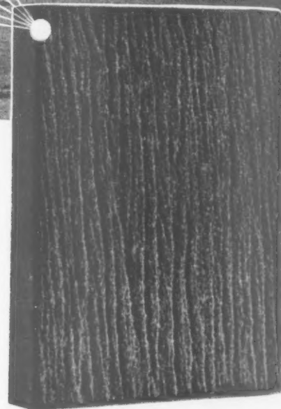
A section of Broughton Moor Stone, showing the distinctive appearance and texture of the frame sawn finish.
