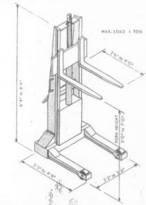
Fig. 15. Typical hand-operated fork lift truck.
