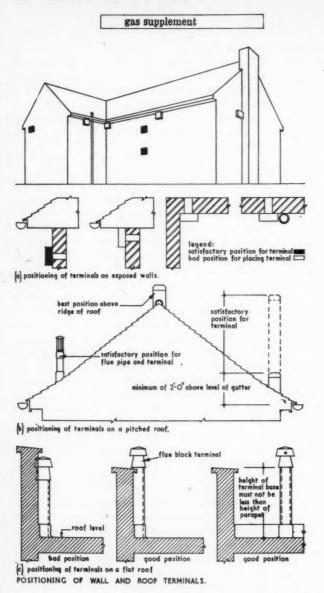
Fig. 2, diagrams showing the correct and incorrect positions of flue terminals.
