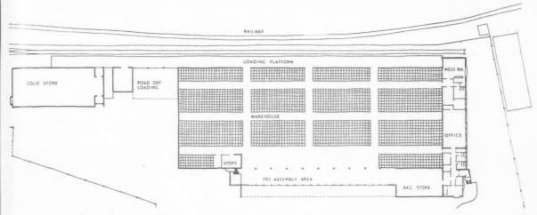
Fig. 3. Perry Barr Warehouse and Distribution Depot of height and span necessary for economical use of mechanical S.P.D. Ltd. Compare with Fig. 2 and note increased equipment.
