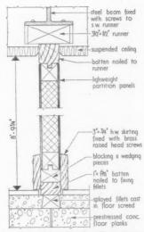
Plan and section at internal wall partition junction with external wall on upper floors |Scale: 2" = 1' 0"]
