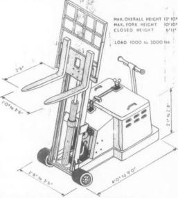
Fig. 16. Typical pedestrian-controlled fork truck.
