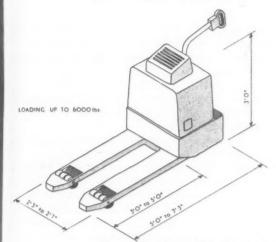
Fig. 12. Typical pedestrian power pallet truck.
