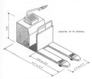
Fig. 13. Typical rider-controlled power pallet truck.
