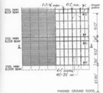
Elevation of external walling to Block B [Scale: #" = 1'0"]
