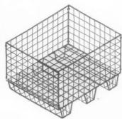
Fig. 10. Collapsible wire mesh box pallet (sometimes called a cage pallet).
