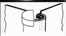
This detail shows the standard arrangement of the hingeing strip-in manganese bronze or other non-ferrous alloy-and the leaves of the door which are in sherardised steel plate or aluminium alloy as required. The hingeing strip has a top cap-shown cut-away. Nothing could be simpler and, nothing is more trouble-free!
