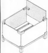
Fig. 9. Detachable sided pallet, can be made in timber or steel.
