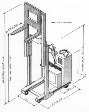
Fig. 18. Typical rider-controlled reach truck.
