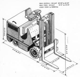
Fig. 17. Typical rider-controlled fork truck.
