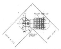
Fig. 20. Turning circle for reach truck. As the forks retract the overall dimension of the truck when travelling is reduced, with consequent reduction in turning circle. Dimensions are again affected by the dimensions of the pallet to be carried.
