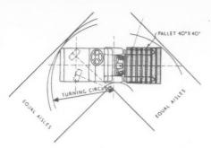
Fig. 19. Turning circle for fork truck. The manner in which the turning circle is determined is indicated in the diagram. The actual dimension depends upon the make of truck and the size of pallet to be carried.
