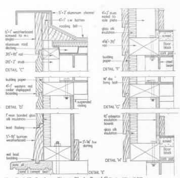
Details A-H of cedar walling to Blocks B and C [Scale: 2" = 1' 0"]
