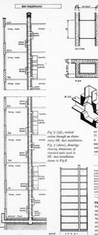
Fig. 8 (right), showing how fresh air is led into an SE. Duct through a horizontal duct at firstfloor level.
