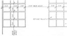
Fig. 21. Typical arrangement of pallets in stacks, showing clearances, and gangway for ordinary fork truck.
