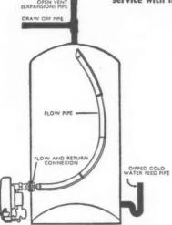
The NEW WORLD Stratalyn is a Regulo-controlled gas water heater for attachment to a storage cylinder or tank by means of a single connexion. It is the GAS application of the IMMERSION HEATER.
