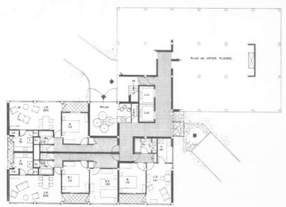
Typical ground floor plan [Scale: 32" = 1'0"]
