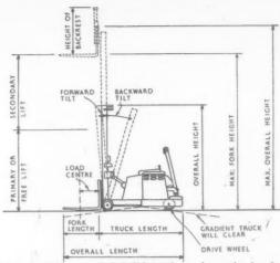
Fig. 14. Diagram of fork lift truck to give main descriptions and dimensions that must be determined when selecting a fork lift truck.
