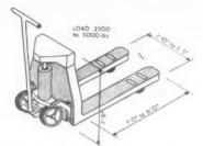
Fig. 11. Typical hand pallet truck.
