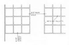
Fig. 22. Typical arrangement of pallets, with reduced gangway for reach truck.
