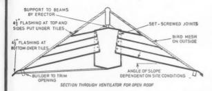
It can be supplied as illustrated for open roofs or with duct and hopper for ceiled roofs. Made in any length in copper, zinc or galvanized steel (painted).
