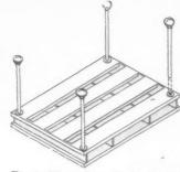
Fig. 8. Tiered flat pallet (a patented design of Fisher and Ludlow).
