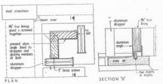
Details of internal corner linings [Scale: 2" - 1' 0"]
