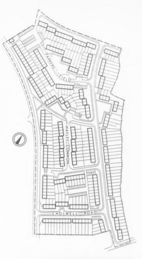
Fig. 1 (below). A typical north to south terrace of houses in the Bandley Hill Scheme. Fig 2 (right). The 16½-acre site laid out at a density of 16 houses per acre.
