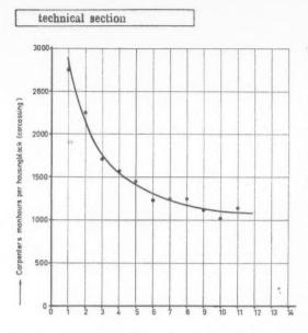
Fig. 5. A graph recording the actual man-hours for carpenters' work as work on the site progressed. Notice the, at first, dramatic improvement in economy as the gangs move from one block to the next. Horizontal figures represent housing blocks.
