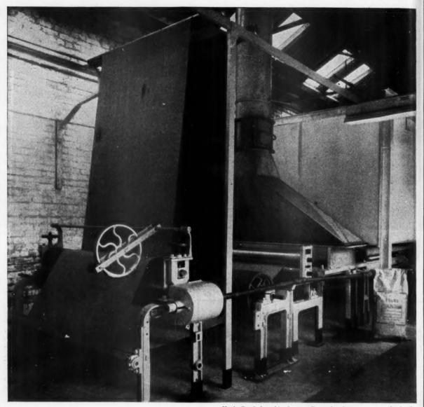
Haul-off end of machine for spreading and curing p.v.c paste on hessian for brattice cloth and on cotton duck for ducting, Machine is at the works of The South Wales Brattice Cloth and India Rubber Co. Ltd., Newport, Mon.
