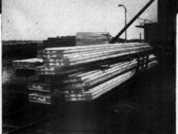
Box beams about to be impregnated with 'Pyrolith'.
