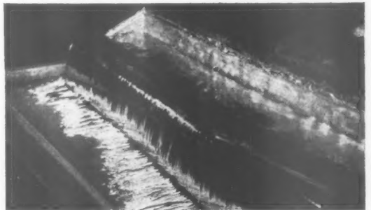
The recasting of sheet lead. Above, a cascade of molten lead is poured on the casting table. Below, lead on the casting table which has cooled and is being cut up into suitably sized pieces. Bottom, lead burning. (Lower photographs by courtesy of MOW).
