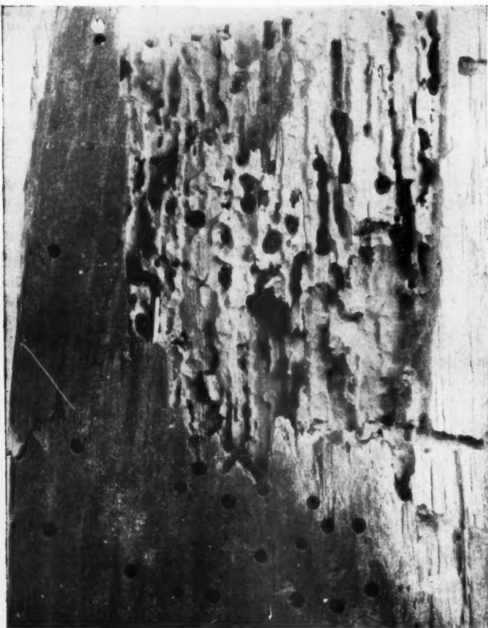
Comparative details of wood attacked, above by furniture beetle, below by death-watch beetle. (Photographs supplied by FPRL.)
