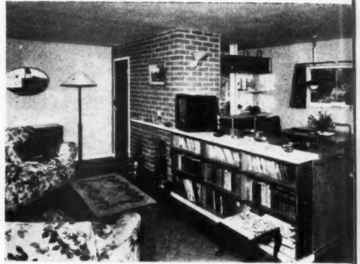
The living room of the house at Great Missenden. Walls and ceiling are plastered, and the floor finish is hardwood block. An existing sideboard had to be used as the basis of the storage unit in the centre of the room.
