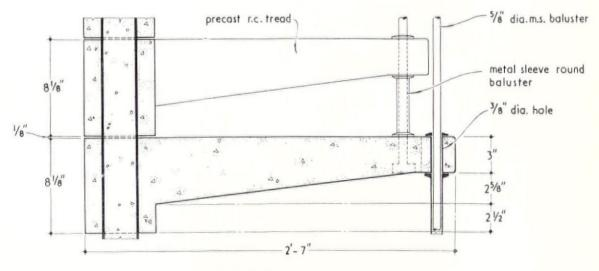
PLAN AND SECTION OF TYPICAL TREAD. scale 1/2 1'0"
