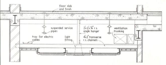
CROSS SECTION OF CEILING. scale 1/2"= 1-0"
