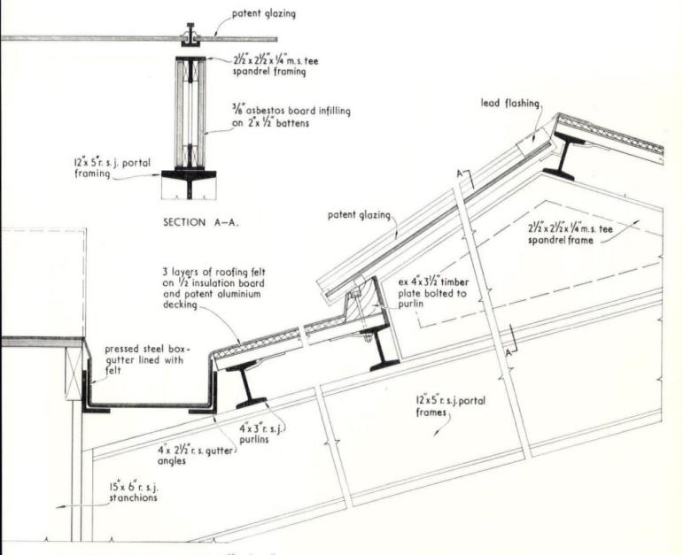
DETAIL SECTION OF ROOF. scale  $1\frac{1}{2} = 1 - 0$
