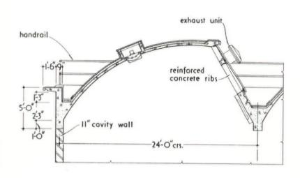
SECTION THRO' BARREL VAULT ROOF. scale 18"=1'-0"
