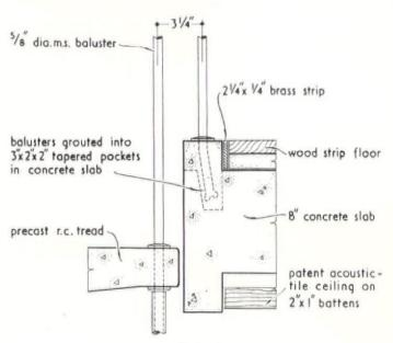
DETAIL AT A - A. scale 1/2" I'- O"
