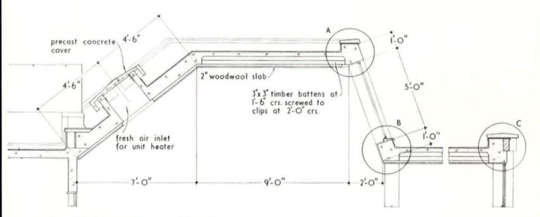
SECTION THROUGH ROOF. scale 1/4"=1'-0"
