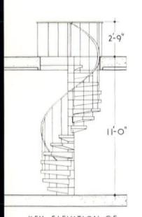
KEY ELEVATION OF STAIRCASE ON X-X scale  $\frac{3}{16}$  =  $\frac{1}{-0}$
