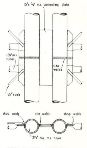
DETAIL OF TYPICAL CONNECTION BETWEEN TRUSSES. scale  $1^{1/2}$  =  $1^{1}$ -O"
