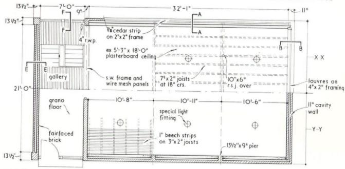
PLAN AT LEVELS X-X AND Y-Y. scale 1/8"= 1'-O"
