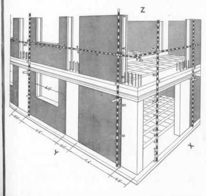
the vertical poles are moved onto the toe of the site slab and these and the horizontal poles are used to check the accuracy of all the major structural parts as the building goes up.
