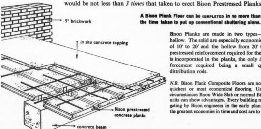
Bison Planks are made in two types-solid and hollow. The solid are especially economical in spans of 10' to 20' and the hellow from 20' to 30'. The prestressed reinforcement required for the total floor is incorporated in the planks, the only in situ rein-
