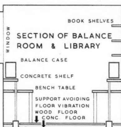
Left; plan of balance room, reference library, storeroom and main entrance (scale: \frac{1}{8} in. = 1 ft.). Above, section of balance room and library (scale: \frac{1}{4} in. = 1 ft.).
