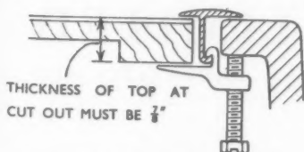
Section through the Twyford wash basin.
