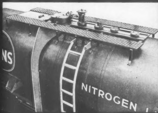
Platforms in rectangular punched Alaflor as supplied to Charles Roberts & Company Ltd., of Horbury Junction, Wakefield. These are fitted to tank wagons built by them for Fisons Limited.
