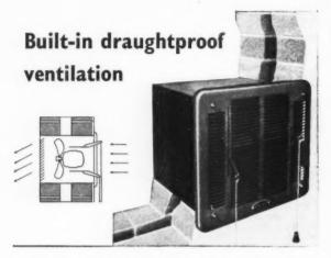
This new draughtproof extract fan is built into the wall. Only a grille inside and outside denote its presence. It comprises a 9in. diam. fan, combined with a draughtprevent shutter, housed in a steel box. The bricklayer fixes the box as easily as an air brick. The fan and shutter unit is inserted afterwards. With this fan you can provide draughtproof ventilation as a built-in feature.
