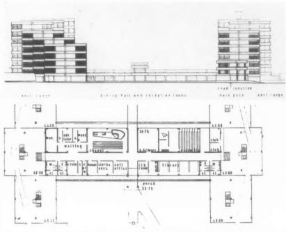
Above, part ground floor plan. Below, long section. Below right, detail plan of residential block.
