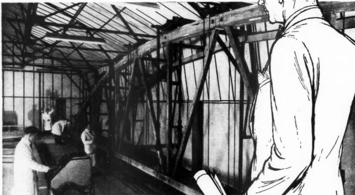
Bowstring truss, 80 ft span, under load test at T.D.A. Research Laboratories.
