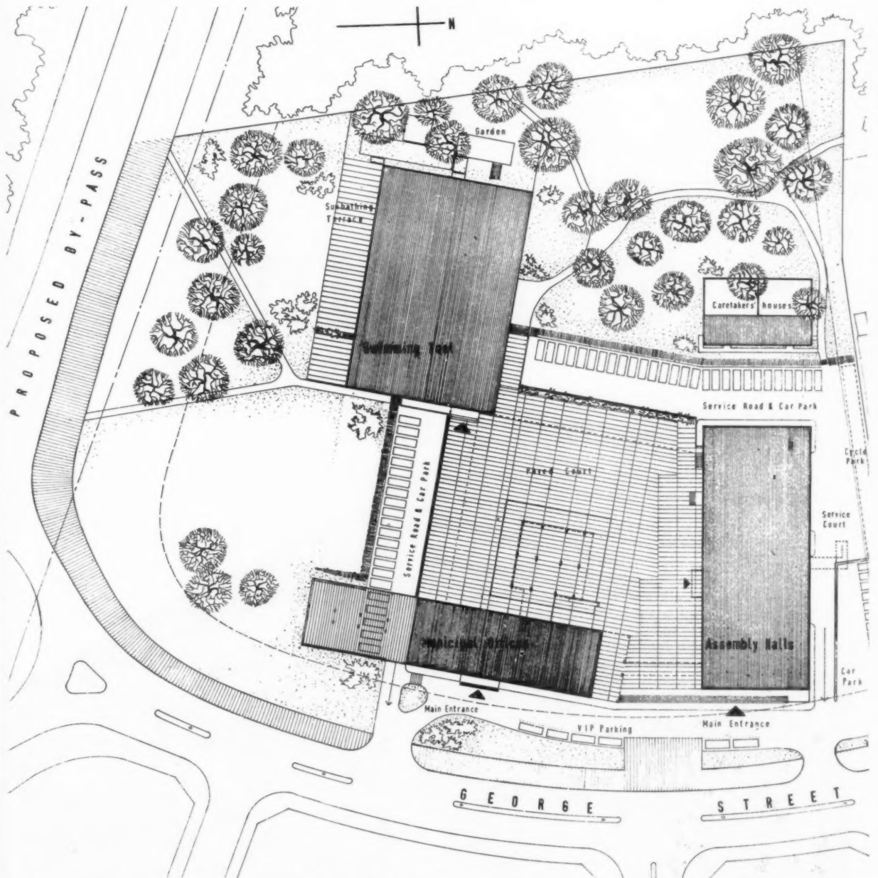
Site plan. A service road runs from the right entrance, past the assembly hall and caretakers' houses, under the swimming pool building and out past the municipal offices.
