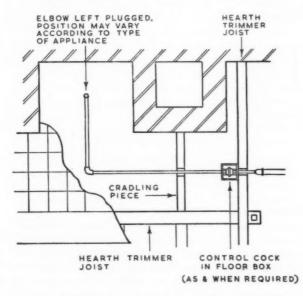
Fig. 17 (b). Concealed connection using normal method.
