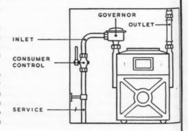
the frictional losses incurred in the pipe installation. The fitting of such a governor will ensure constant pressure conditions throughout the premises, see Fig. 4. In built up areas where it may be expected that the working pressure in the mains will be normal low pressure (4 in.-8 in. w.g.) and undue variations unlikely, individual appliance governors, small and compact, are often utilised, either as an integral part of the appliances or fitted adjacent thereto.
