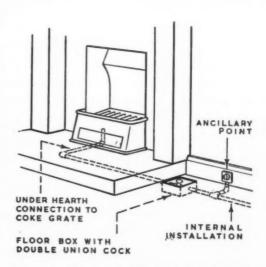
Fig. 20. Provision of an ancillary point on skirting board.
