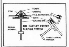
alloy construction; with new glazing Aluminium new shape with new glazing system to admit far more light; absence of internal supports for unrestricted working space; virtual elimination of breakages—each pane is enclosed on all edges by P.V.C. extrusion and aluminium frame, and so safe-guarded against shock, draughts and weather, and against break-ages caused by expansion and contraction; stove enamelled struc-ture preventing unsightly surface
