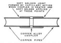
Fig. 2 (a) (above). Copper pipe and capillary joint.
