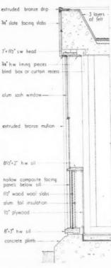
Section through external wall in single-storey block [Scale: ]" = 1' 0"]
