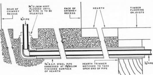
Fig. 17 (a). Concealed connection using sleeve method.
