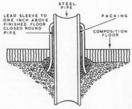
Fig. 14. Lead sleeve protection for steel pipes in composition floors.
