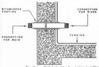
Fig. 3 (c). Method of entry where tanking is employed in basement of block of flats. A flange is welded on a short length of pipe which is coated with bituminous material and set in position before concrete is poured.
