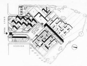
Site plan, with phase one hatched; Nos. 2 and 3 indicate second and third phases  $\,$
