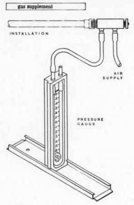
Fig. 22. Pressure testing set.
