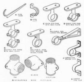
Fig. 13. Types of pipe fixings and fittings.
