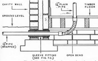
Fig. 8 (b). Method of service entry where pipe can be withdrawn and replaced.
