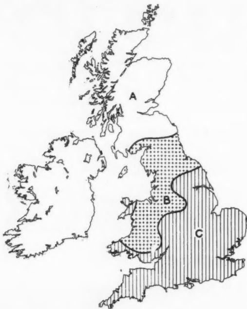
Fig. 6. Suggested areas where control of solar radiation is necessary. Area A: no control necessary. Area B: control required where glazing to wall ratio exceeds 65 per cent. Area C: control required where glazing to wall ratio exceeds 55 per cent.
