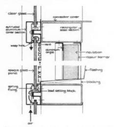
Fig. 9. Reduction of surface temperature of panel by ventilation of cavity.
