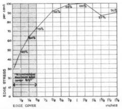
Fig. 10. Variation of tensional edge stress in glass with edge cover indicating the need for minimal edge cover. (From T. A. Markus, "The Glass Curtain Wall.")
