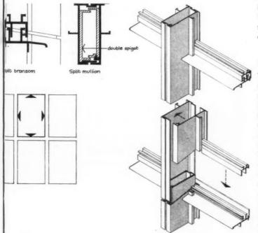
Fig. 4. Thermal movement in metal framing type B. Male and female sliding mullions and transoms. (Holoplast.)
