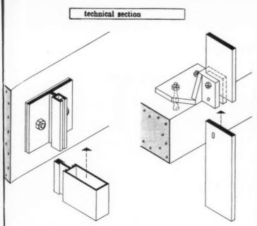
Fig. 1. Allowance for thermal movement between framing and structure. Left, sliding joint (BSC Ltd., Vistalite); right, bolt and slot joint (J. Williams & Sons Ltd.).
