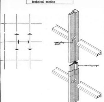
Fig. 3. Thermal movement in metal framing type A. Sliding joints between mullions and transoms. (Templewood Hawksley.)
