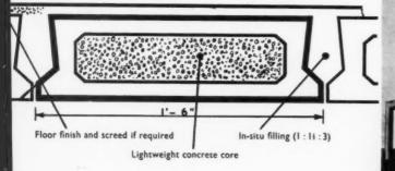
Precon manufacture a complete range of flooring. A distinctive feature of Precon flooring units is that the core is made of lightweight concrete to give excellent sound and heat insulating qualities.
