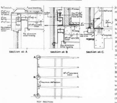
Fig. 11. Spring-loaded joints between cladding and structure to accommodate deflection of structure (College of Further Education, Ystrad Mynach. Architects, Alwyn Lloyd and Gordon. Cladding by J. Williams & Sons Ltd.)
