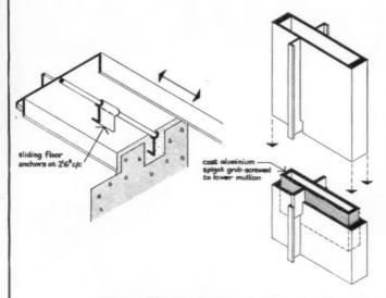
Fig. 2. Allowance for thermal movement. Left, movement between cill and structure; right, movement in mullion (note weathering of spigot). (Williams & Williams Wallspan.)
