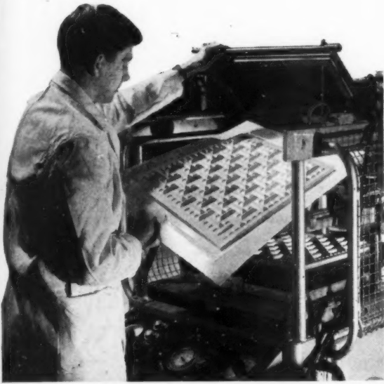
Vacuum forming panels in 'Flovic' vinyl copolymer sheet in the T.S. and D. Dept. Laboratories, I.C.I. Plastics Division.
