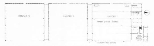
Fig. 3. Plan of the hangar. Hangars 2 and 3 will be erected at a later date. Spaces between hangars will be used for workshops.
