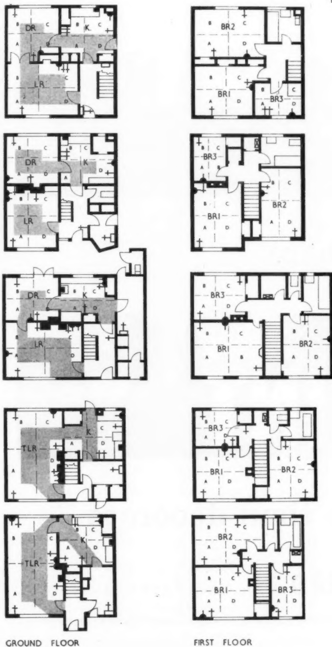
Fig. 1. Plans of the five house types surveyed showing the existing and recommended electrical provision. Shaded areas in ground floor plans are areas where appliances were seldom found.
