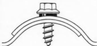
A. Type self-tapping screw with neoprene washer for seams in metal sheeting.
