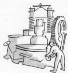
As well as making top quality sand lime, concrete and refractory bricks, the Sutcliffe, Speakman Emperor Press makes bricks from clinker, burnt shale, slag, etc. – once considered useless waste. They're good quality bricks, consistent and always well formed.
