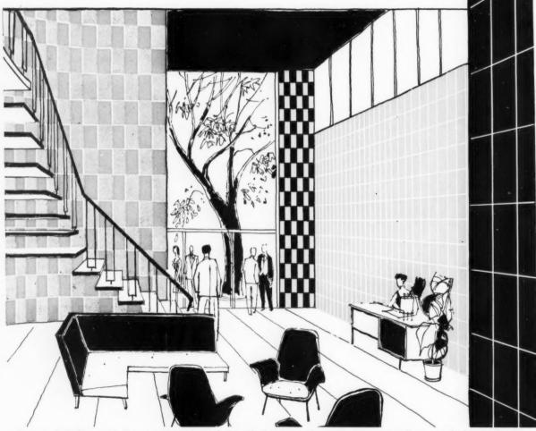
In new buildings and the reconstruction of old, Marleymura tiles make an outstanding practical contribution to functional wall decoration. MARLEYMURA TILE SIZES, the actual dimension of each tile is 12"x 5 1/8" which permits any design to be used while still maintaining an equal 1/8" framed spacing between tiles. Five pastel colours and black, gauge jointed in white.
