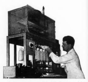
Equipment used at the T.S. & D. Department, I.C.I. Plastics Division, to measure the "creep" characteristics of 'Perspex' acrylic sheet.
