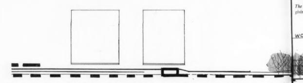
An east-west section through Gloucester Green, with office blocks towering over the transport centre on the left, the core road show broken line running past Worcester College and running beneath the Gloucester Green redevelopment. At Gloucester Green is a pell platform with garages below for 1,500 cars. Shops, offices, an hotel and entertainment centre rise through the deck and form a co of open and covered squares.
