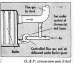
G.A.P. conversion unit fitted to sectional boiler for Central Heating.
