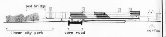
An east-west section through the city core at Carfax, showing the pedestrian ramp, the memorial (see plan overleaf), the sunken road, garages, and the pedestrian platform with commercial buildings over.
