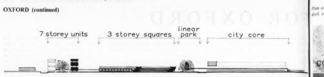
Section AA, showing, from left, the proposed school, the seven-storey maisonette blocks, the residential squares, and the pedestrian ramping the linear park leading over the sunk core road to the shopping and commercial core with car parks under.
