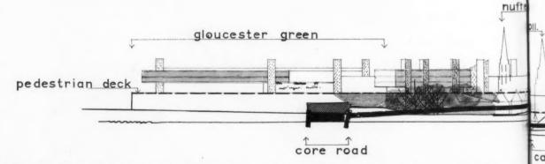
The west elevation of the new core, showing the pedestrian deck on the left, a section through the core road, Nuffield Colle Castle Mound and the towers of offices above the pedestrian deck as it runs south, fronted by a linear park, to Christ C
