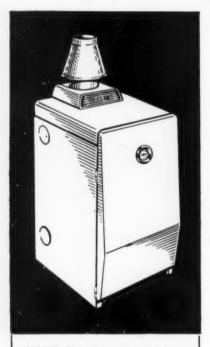
MODEL SA 45 has an output of 45,000 B.T.U.'s constant loading suitable for up to 9 radiators (220 sq. ft. surface) and 30 gallons of hot water. Maximum fuel consumption 3 pints per hour.
