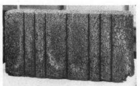
Fig. 4. Grooved partition block.
