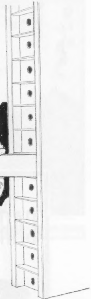
The cellular core of Gypunit Panel permits the easy insertion of wood blocks to accommodate fastenings for door frames, glazing openings, etc.
