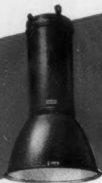
GEAR INCORPORATED. For high-bay installations. Control gear housed in the fitting. Robust steel canopy contains choke, power factor correction capacitor. Reflectors: standard overlamp type, finished Simplex 'Arvit' (acid resistant vitreous enamel). £18 1s. 4d. 250W £18 4s. 4d. 400W
