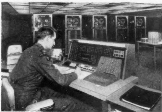
The computer itself is a series of units linked together by under-floor cables, and controlled from a central desk, left
