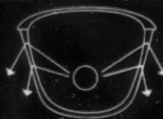
Refraction by machined 'Perspex' refractor plates designed to give most efficient light distribution.
