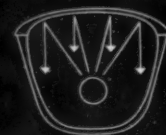
Reflection from Opal 'Perspex' canopy — over 80%.
