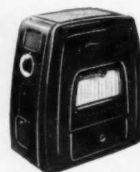
"ESSE" AUTOVECTOR heating stove incorporates a fuel hopper and thermostatic control. For heating lounges, bars and reception rooms
