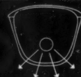
Transmission through base of clear 'Perspex' bowl — 90%.
