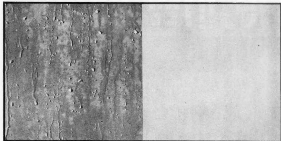
Actual photograph showing panel with left hand side painted with first quality Emulsion Paint and right hand side with ANTICON and then subjected to severe condensation conditions.
