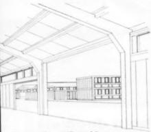
The range of new "Alborough" prefabricated concrete portal frame factory buildings and two storey office blocks are available in a wide range of structures, adaptable to meet individual requirements.
