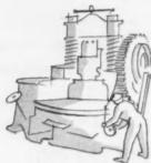
As well as making top quality sand lime, concrete and refractory bricks, the Sutcliffe, Speakman Emperor Press makes bricks from clinker, burnt shale, slag, etc. – once considered useless waste. They're good quality bricks, consistent and always well formed.
