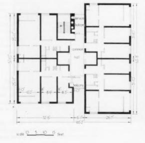
Plan of typical upper floor, structural walls shown in solid black
