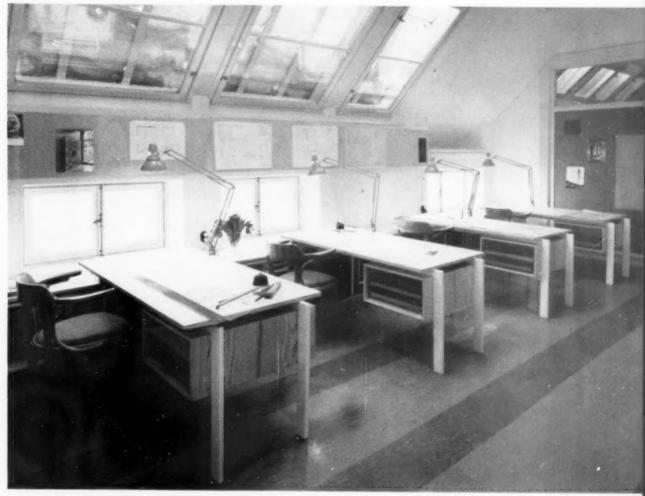
These ingenious drawing tables in an architect's office are designed to rest, at one end, on a continuous sill. There is no table top, since this is provided by the drawing board itself. Instruments are held in a narrow container on the window side and reference books are placed either on the sill or on tray-type drawers on the room side.
