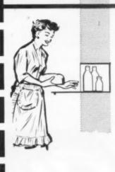
Here's an idea that pays for its space. The Beacon Delivery Hatch, simply built into the wall, is hygienic, thief-proof, labour saving and neat. It helps the roundsman and the housewife... this is how it works... Once the roundsmen close the outside doors they lock automatically. The housewife opens the inside door and removes the goods which have kept clean, cool and safe from pilfering. When this is done the outside doors are unlocked ready for the next delivery.
