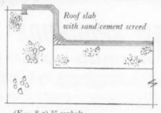
$(K=8\cdot5)\,\frac{3}{4}''$  asphalt  $(K=9\!\cdot\!0)\,4''$  sand/cement screed  $(K\!=\!\text{10}\!\cdot\!0)\,6''$  normal structural screed
