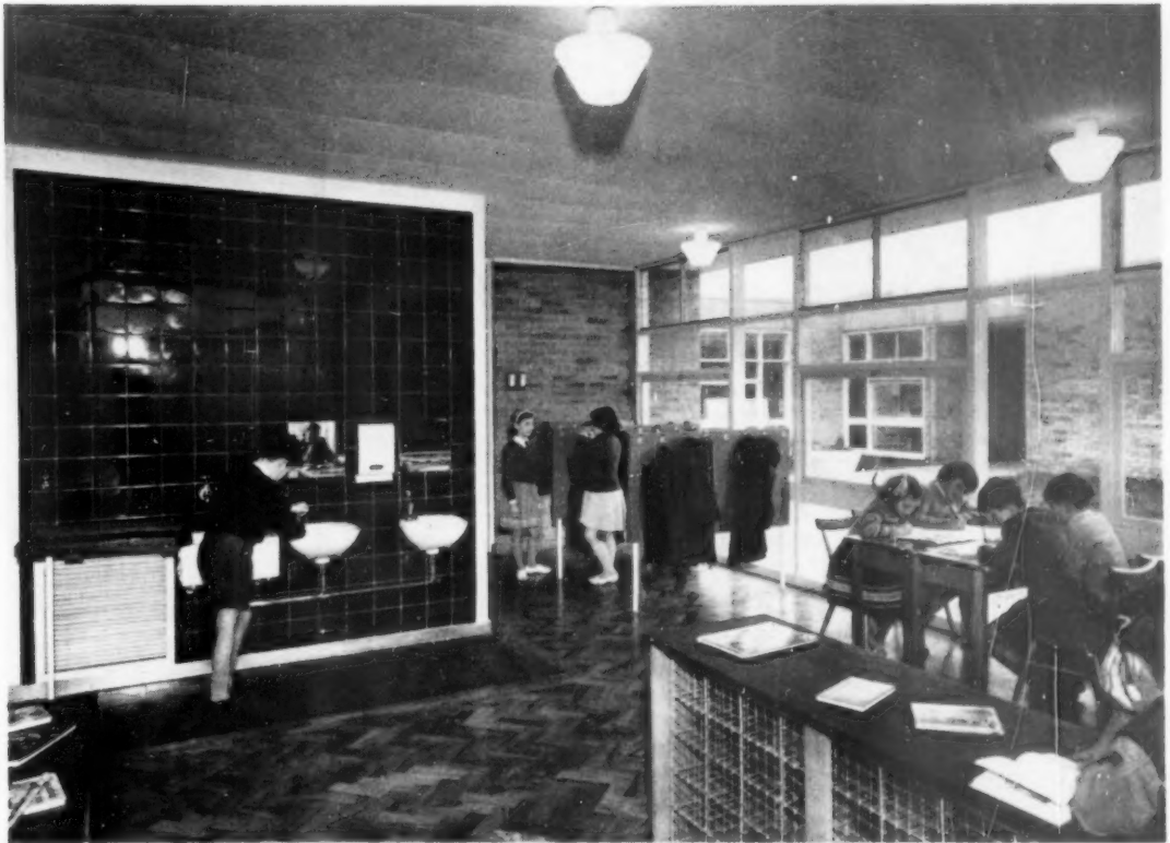
Following standard practice in Herts for primary schools, in each classroom the heating, plumbing and teacher's storage are grouped together into one compact unit between the main teaching space and the cloaks/practical area
