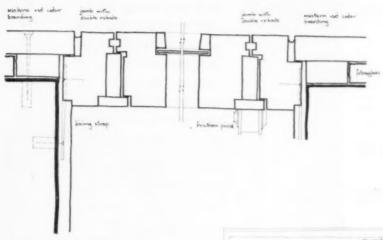
Plan through jamb of window below friction pivot, above left, and plan through jamb of window above friction pivot, above right
