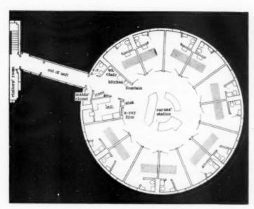
Plans of the rectangular and circular ward units which were used for the Rochester experiment
