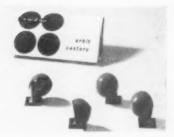
Orbit furniture castors, designed by Joseph Gillott & Sons Ltd., in conjunction with R. David Carter, M.S.I.A., made of zinc base alloy and mild steel with stove enamelled finish, enclosed bearings and sealed-in lubrication: "such small components are of importance and are often overlooked... often the appearance of a chair is ruined by ugly castors."
