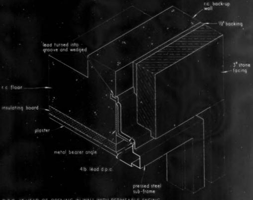
D.P.C. AT HEAD OF OPENING IN WALL WITH PERMEABLE FACING
