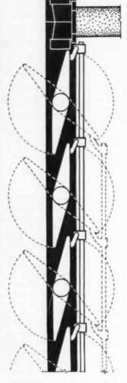
HOPE'S Sunbreakers are made in. a variety of profiles in pressed steel or aluminium, both single and double skinned, fixed and movable: the latter can be hand or mechanically operated.
