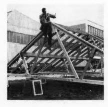
by bolting up the bottom tie bar and nailing a collar, and costs less than the two orthodox trusses it is designed to replace. Standard pitches are 22½, 30 and 35 degrees, with spans up to 36 feet. No change in technique is necessary, as the roof construction remains normal. (Dexion Ltd., 65, Maygrove Road, Kilburn, London, N.W.6.)
