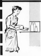
Here's an idea that pays for its space. The Beacon Delivery Hatch, simply built into the wall, is hygienic, thief-proof, labour saving and neat. It helps the roundsman and the housewife . . . this is how it works . . . Once the roundsmen close the outside doors they lock automatically. The housewife opens the inside door and removes the goods which have kept clean, cool and safe from pilfering. When this is done the outside doors are unlocked ready for the next delivery.
