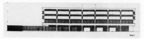
West elevation (above) and section (right). Reading areas in this design are largely concentrated in the double-height reading room with glazed roof over. The assessors felt there were disadvantages, chiefly of noise and disturbance because of this grouping
