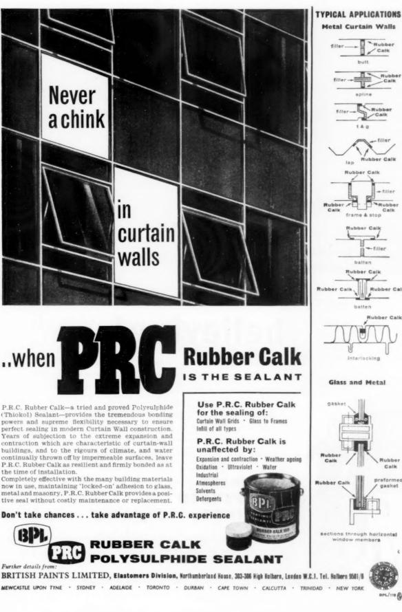
Rubber Calk batten Rubber Calk interlocking **Glass and Metal** Rubber Calk
