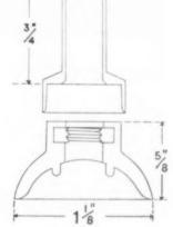
The protruding bolt end is given protection from corrosion by the Selacap, even under the worst possible weather conditions, thus keeping the roof sheets free from rust stains.
