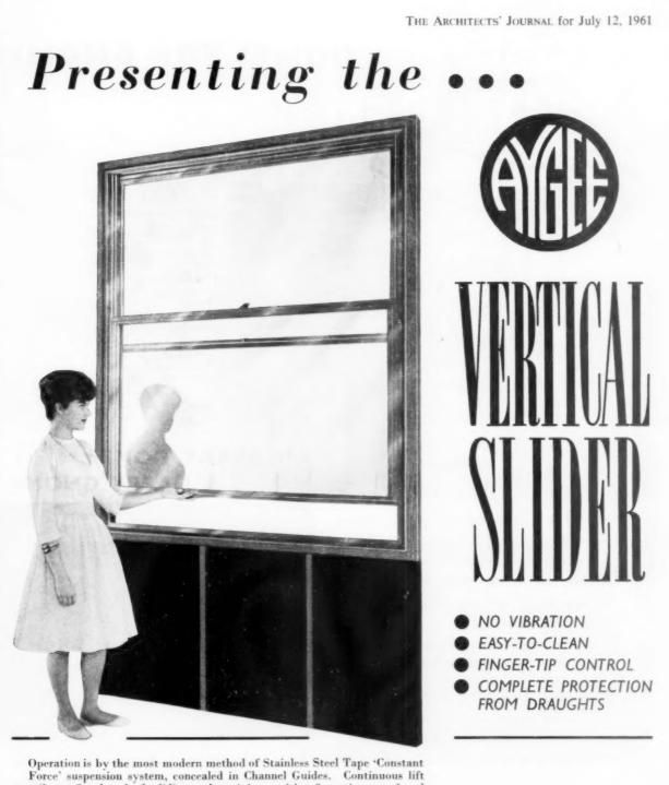
Operation is by the most modern method of Stainless Steel Tape 'Constant Force' suspension system, concealed in Channel Guides. Continuous lift rails are fitted to both sliding sashes giving positive fingertip control and allowing either sash to be held in any desired position. Both sliding sashes are double 'Weatherstripped' with Silicone treated wool pile, and the top, bottom and meeting rails are 'Weatherstripped' with cushioned P.V.C.
