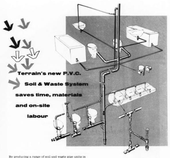
unplasticised P.V.C., A. B. Plastics Ltd. have now made possible a new system that makes full use of the many advantages of this material while also saving time and labour.
