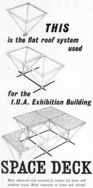
This patented system provides for a wide range of cladding and suspended ceilings, allowing the greatest scope and flexibility of roof design, while maintaining maximum strength and internal capacity.
