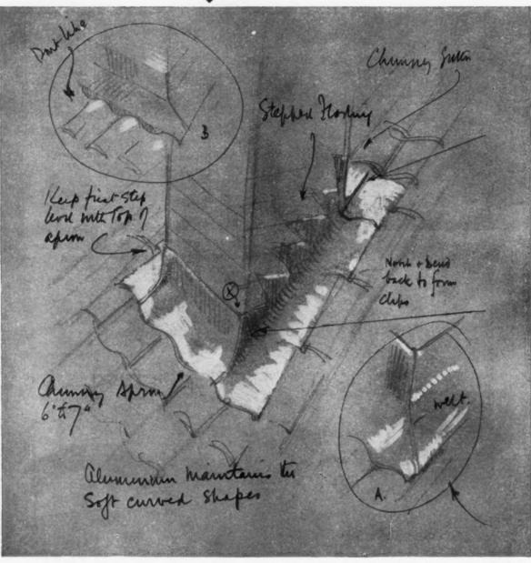
Architect's drawing of flashing with notes
