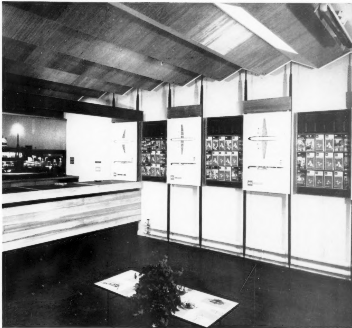
This series of panels, mounted on verticals fixed to floor and ceiling, creates a flexible and demountable method of display.
