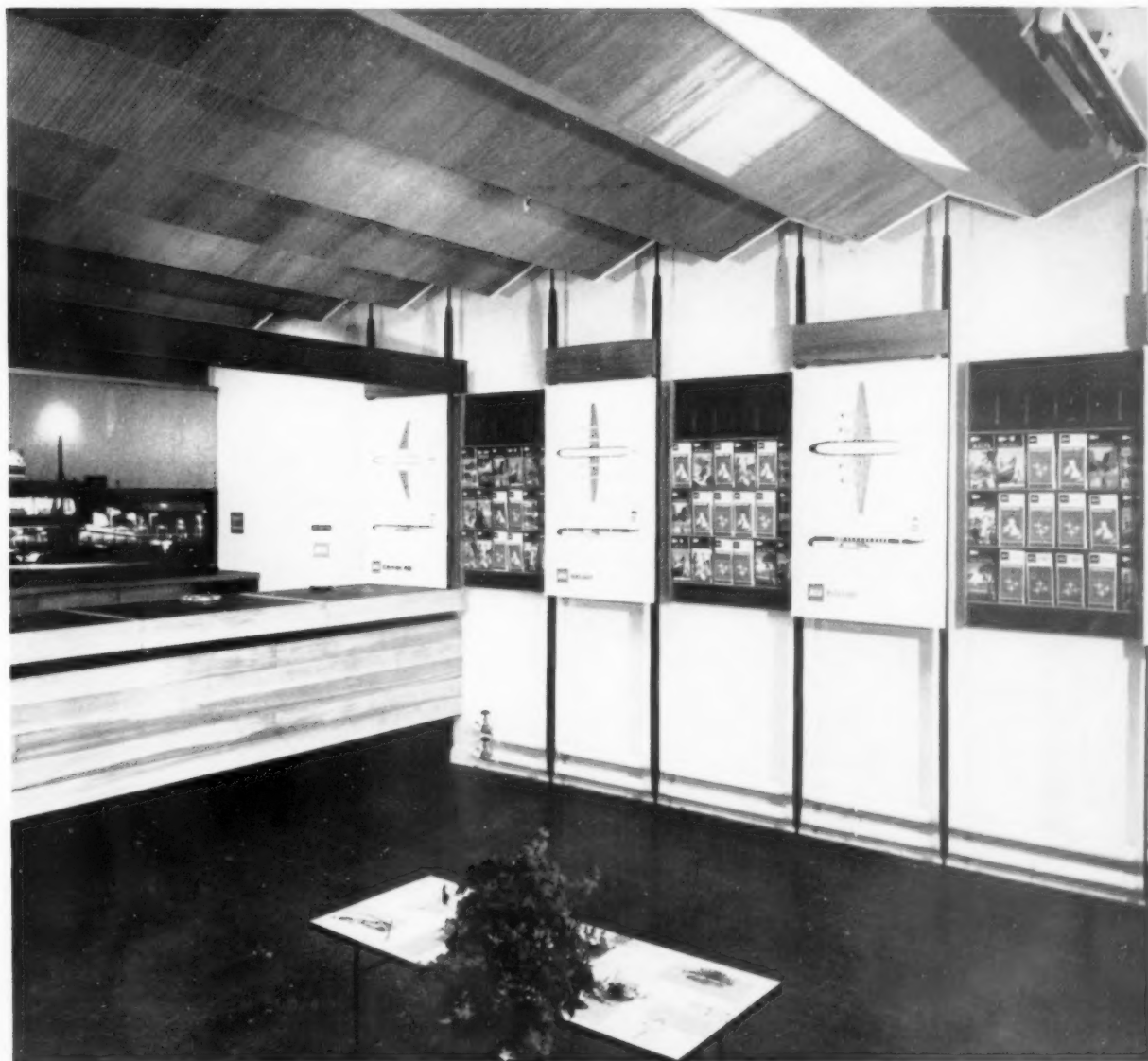
This series of panels, mounted on verticals fixed to floor and ceiling, creates a flexible and demountable method of display.
