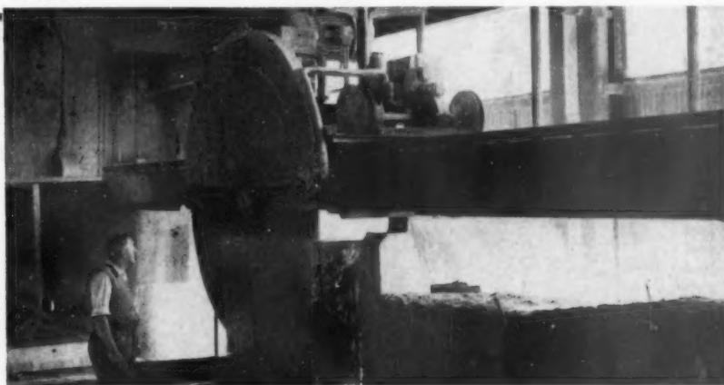
An 11-ft.-diameter primary cutting saw sawing through rough stone which is carried on cars
