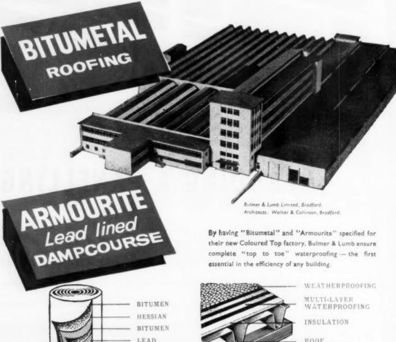
"Armourite" Dampcourse, reinforced with a lining of sheet lead, gives that "extra" protection required in good class building construction.
