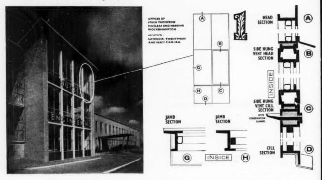
The Architect has achieved a bold elevational effect by setting Steel windows, between the verticals and horizontals of his concrete structure — the result has many of the advantages of curtain walling but avoids the usual flat effect.
