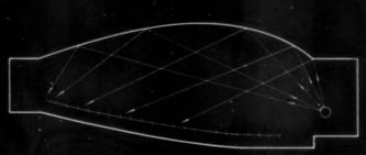
A GOOD REFLECTING CEILING (longitudinal section)
