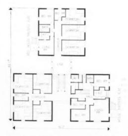
First floor plan of typical residential block [Scale: 30" = 1' 0"]
