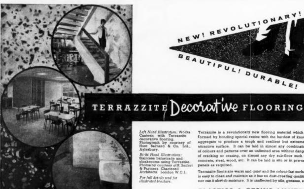
Terrazzite is a revolutionary new flooring material which is formed by bonding special resins with the hardest of known aggregate to produce a tough and resilient but extremely attractive surface. It can be laid in almost any combination of colours and patterns over an unlimited area without danger of cracking or crazing, on almost any dry sub-floor such as concrete, steel, wood, etc. It can be laid in situ or in pre-cast
